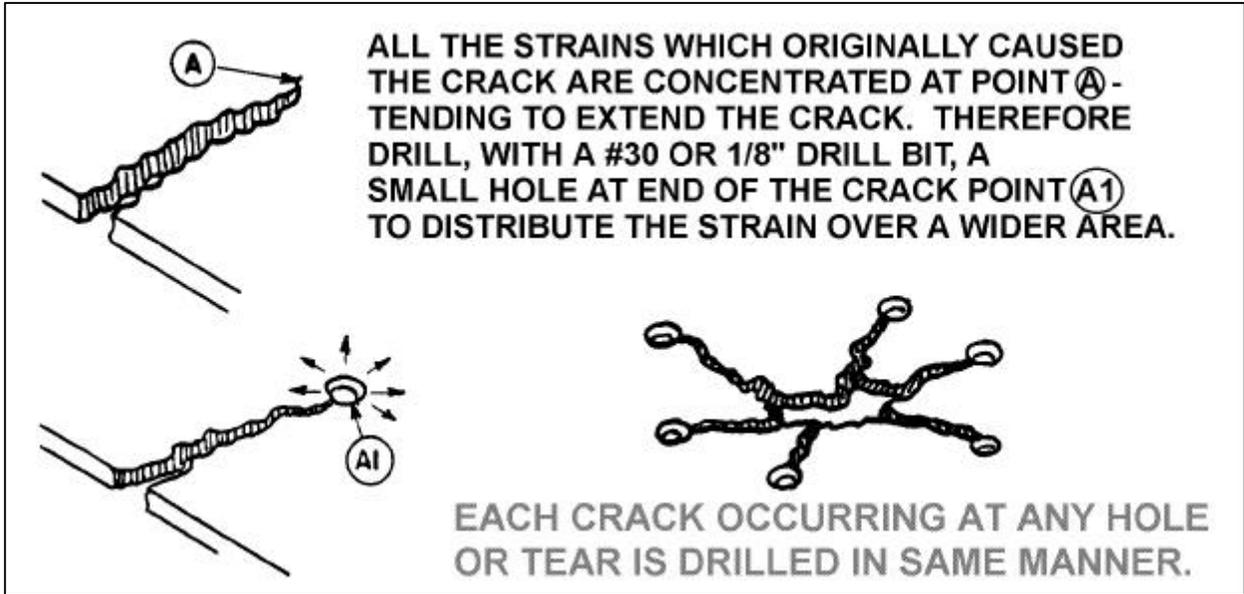
FIGURE 3-21. Stop-drilling cracks.
