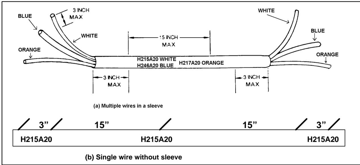
FIGURE 11-23. Spacing of printed identification marks (direct marking).
