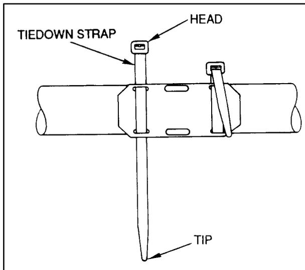
FIGURE 11-29. Tie-down strap installation.
