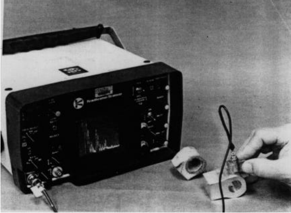
FIGURE 5-17. Typical portable ultrasonic inspection instrument.
