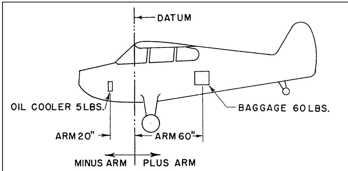
FIGURE 10-2. Illustration of arm (or moment arm).
