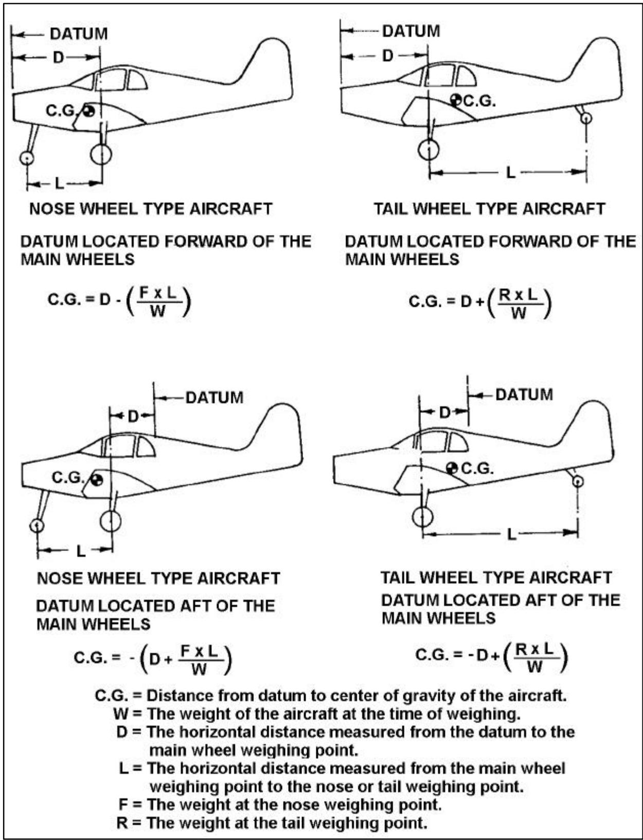
FIGURE 10-4. Empty weight center of gravity formulas.
